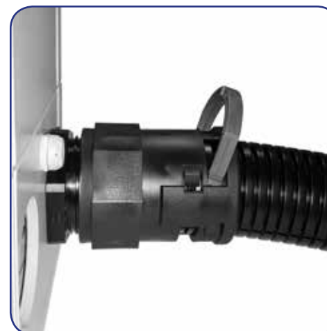
These clips are located within the gland body and lock across the helix in the conduit
